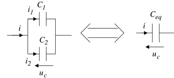
$$i = i_1 + i_2 = C_1 \frac{du_c}{dt} + C_2 \frac{du_c}{dt} = (C_1 + C_2) \frac{du_c}{dt}$$
