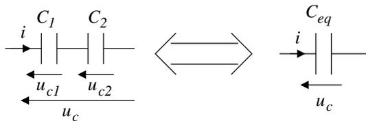
$$u_c = u_{c1} + u_{c2} \Rightarrow \frac{du_c}{dt} = \frac{du_{c1}}{dt} + \frac{du_{c2}}{dt} = \frac{i}{C_1} + \frac{i}{C_2} = \left( \frac{1}{C_1} + \frac{1}{C_2} \right) i$$
